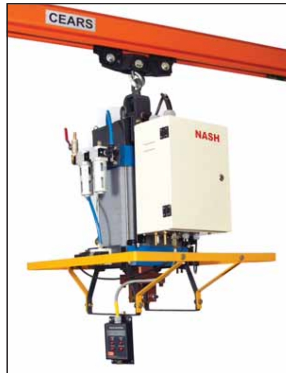
150 KVA Transformer with NASH-NAD 700 Controller Mounted - Asian Design
