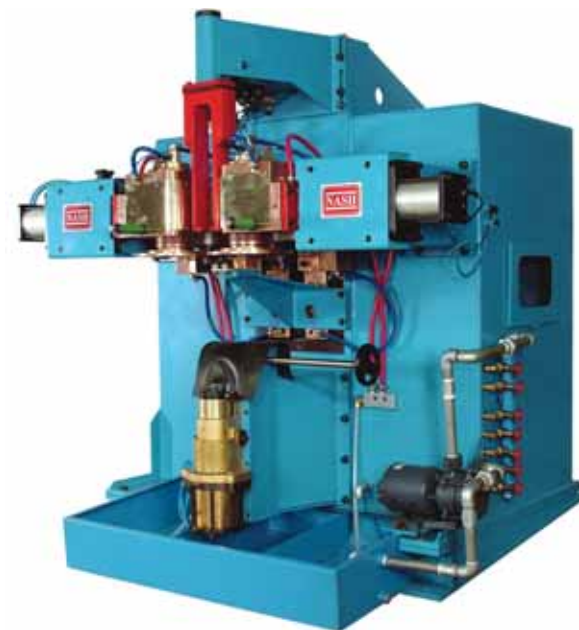
150 KVA Special Purpose Seam Welder for Strut and Shock Absorber Assembly
