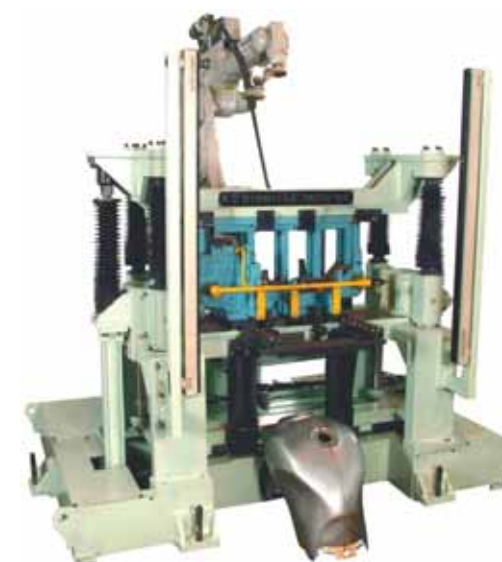
Robotic Welding Automation for Fuel Tank
