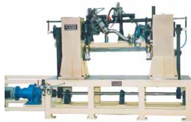
Horizontal SPM for circular welding of exhaust converter
